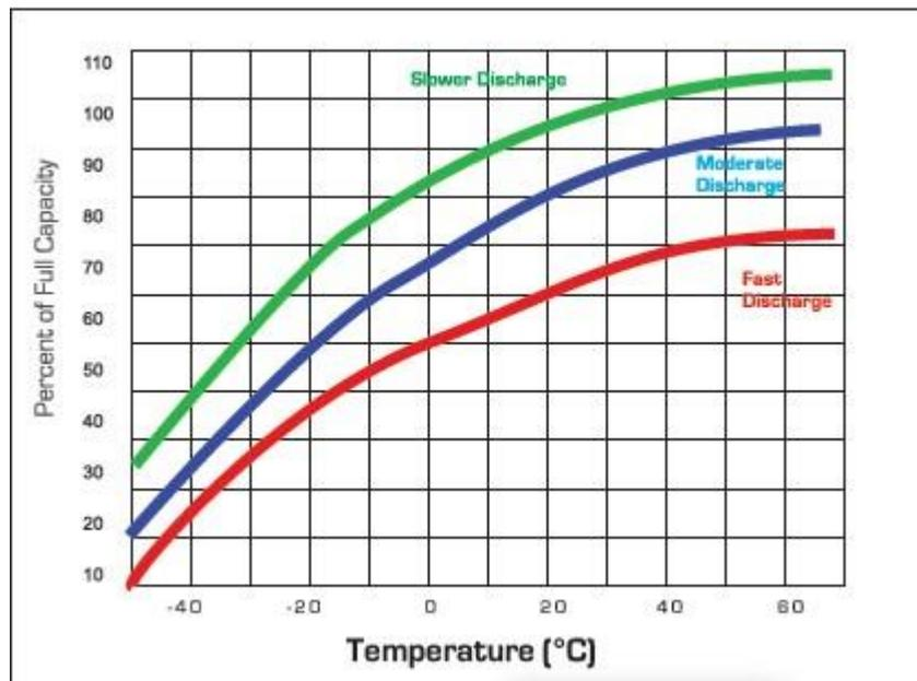
The above graph shows how the performance of Lead Acid batteries varies at different temperatures. If the temperature in the battery is very low (Red curve). Then battery discharge at a faster rate. And if the temperature of the battery is in between the ambient temperature then the battery discharge at moderate rate and if the temperature is above 30 Degree that mean battery performs well.
